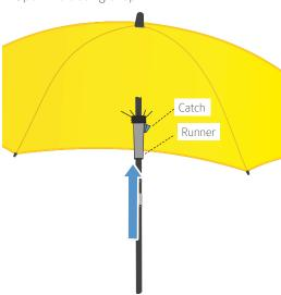
> Keep parasol away from you, press catch and > Press catch and push runner down push slider upwards. The parasol spreads out > Secure parasol with fastening strap and the runner engages in the upper position. Due to the size of the parasol, this may require a little more strength
